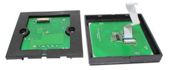
3. Fix the base of controller in the  $86\times86$  installation box (customers need to buy the installation box by themselves) on the wall with screws.
